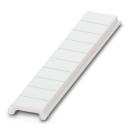
Zack Marker strip, flat, can be ordered: Strip, white, labeled according to customer specifications, mounting type: snap into flat marker groove, for terminal block width: 3.5 mm, lettering field size:  $3.5 \times 5.2 \text{ mm}$ , Number of individual labels: 10
